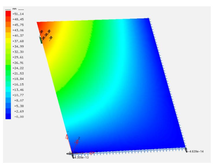
Figure A 10 mm thick panel showing about 50 mm deflection
